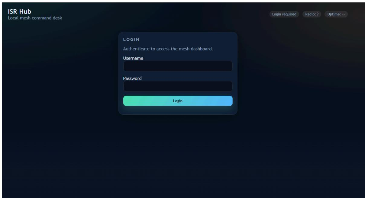
The hub implements a simple single-user authentication model suitable for a local, offline system. Login is handled via `/auth/login`, which verifies credentials against a password hash generated using Python's standard library `scrypt` implementation. This avoids the need for heavy native dependencies while still providing a memory-hard key derivation function.
