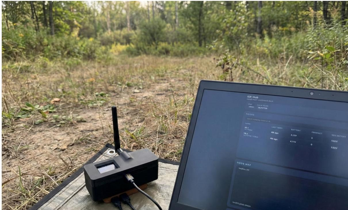
The goal of this project was to build a small, self-contained mesh communications and sensing system that can operate without any external network infrastructure. The system is designed to demonstrate how low-power, long-range radios can be combined with local web technologies to collect, relay, and visualize data from distributed devices. A key requirement is that the system remains fully local and offline, while still being accessible from common user devices through a standard web browser.
