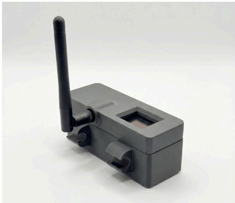
The T-Beam enclosure was designed as a snug, tool-free protective shell that clips together without screws or external hardware. The internal geometry closely follows the T-Beam PCB, ensuring the board is held firmly in place and protected from movement or impact. The enclosure is printed in ABS and avoids thin, unsupported features, which makes it mechanically strong and resistant to cracking. It has been drop tested and is robust enough to survive typical handling and accidental drops.
